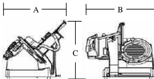
**Product Table:** Full gravity feed 45° angle with articulating rear mounted pusher that runs the entire length of the table to secure product for increased yield and consistency in every slice. A fence is provided for holding small products.
