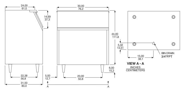
NOTE: Allow 6" minimum space at back for ice machine ventilation and utility connections.
